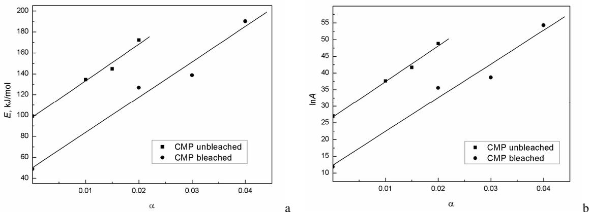
Figure 5: Linear dependences of: (a) the activation energy,  $E$  (kJ/mol) and (b) the preexponential factor,  $\ln A$ , on the extent of process development,  $\alpha$
