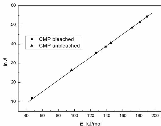
Figure 6: The compensation effect: linear dependence of  $\ln A$  vs  $E$ , kJ/mol
