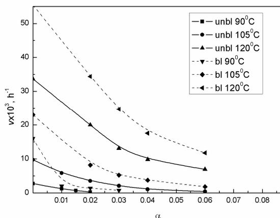
Figure 3: Dependence of the current rate,  $v$  ( $\text{h}^{-1}$ ), on the extent of process development,  $\alpha$ , at the temperature values studied for bleached (-----) and unbleached (—) CMP
