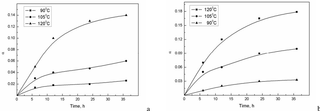
Figure 1: Kinetic curves of increase of the ageing process extent for: (a) unbleached CMP; (b) bleached CMP
