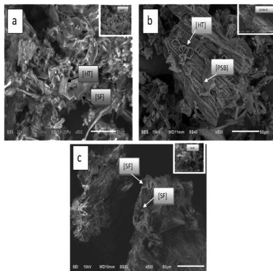
Figure 2: SEM images of pineapple residues; a: shell, b: leaf bracts and c: core (HT: helical tracheid; SF: sclerenchymatic fibre; PSB: plate-shaped bundles)
