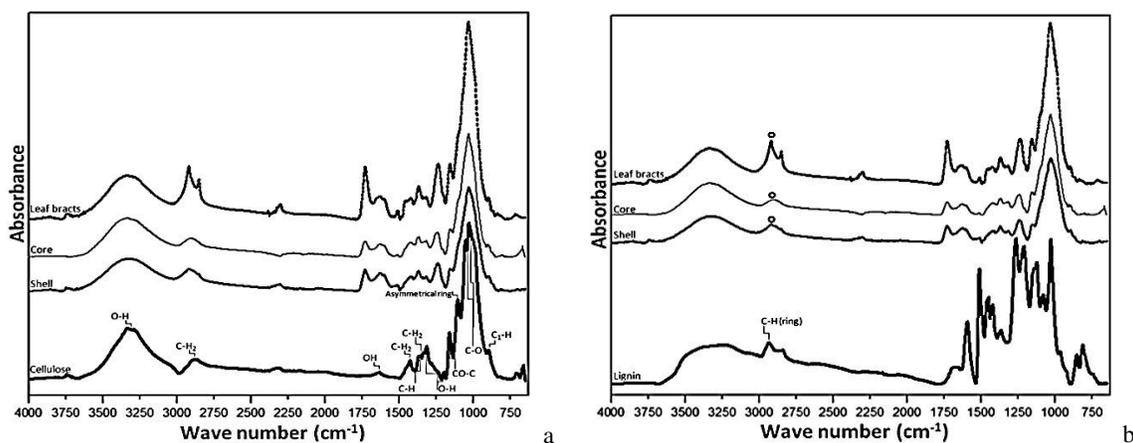
Figure 1: FTIR spectra of pineapple residues in the 4000-750  $\text{cm}^{-1}$  range in comparison with the spectra of (a: cellulose, and b: lignin)
