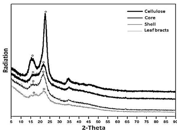
Figure 3: X-ray diffraction profiles of pineapple residues in comparison with the diffraction pattern of a commercial preparation
