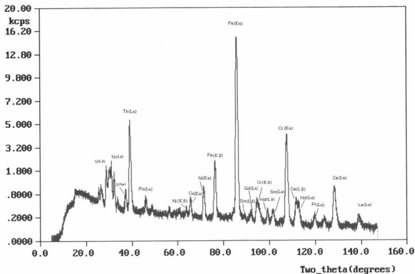
Figure 6: XRF of functional filter paper-REEs complexes
