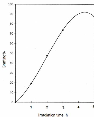
Figure 1: Grafting % vs radiation time, h, for grafting of acrylonitrile 45% monomer concentration onto Whatman filter paper (W1) at 4 kGy/h dose rate
