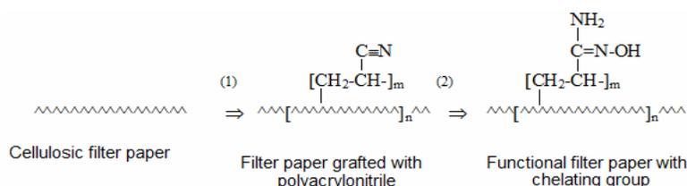
Scheme 1: Filter papers grafted with polyacrylonitrile (90% grafting ratio) and treated with hydroxylamine ethanol solution at 70 °C for 2 h
