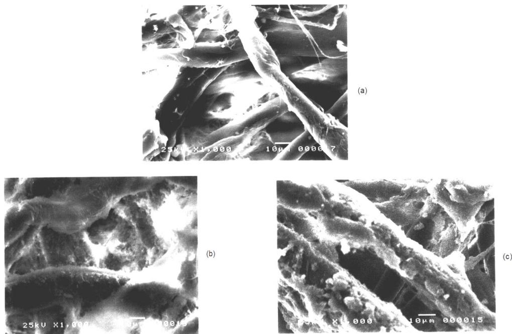
Figure 4: SEM of (a) filter paper, (b) grafted filter paper and (c) functional filter paper
