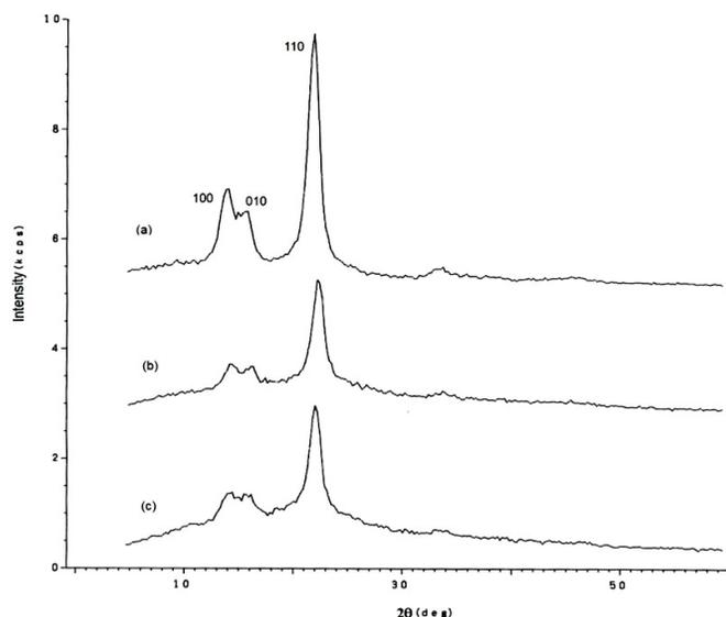
Figure 3: X-ray diffraction of (a) filter paper, (b) grafted filter paper and (c) functional filter paper
