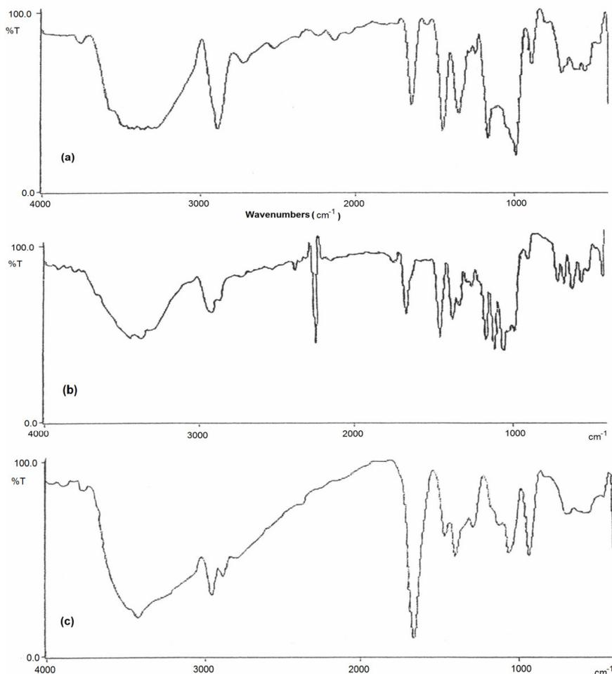
Figure 2: FTIR of (a) filter paper, (b) grafted filter paper and (c) functional filter paper
