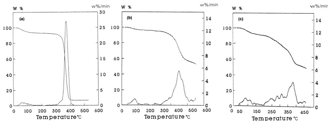
Figure 5: TGA of (a) filter paper, (b) grafted filter paper and (c) functional filter paper
