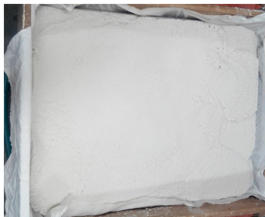
Figure 6: NFC prepared from cotton linter pulp
