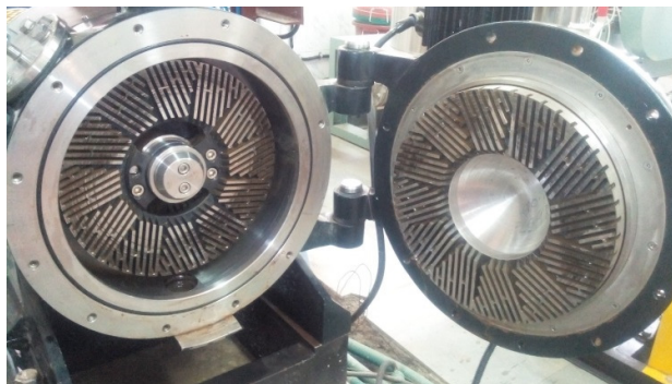
Figure 2: Tri-Disc Refiner (TDR) opened to show the refining surfaces
