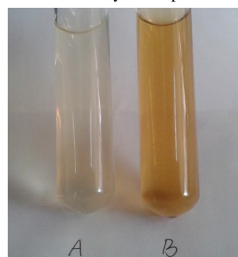
Figure 4: Extraction solutions before and after treatment by resin; A) Resin-treated ES; B) Original ES
