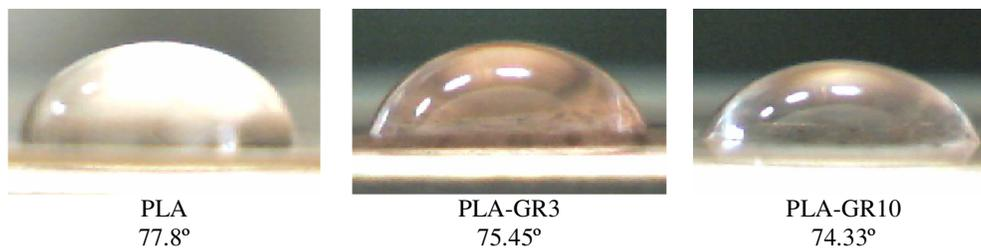
Figure 2: Water contact angle of neat PLA and PLA/grape seed biocomposites
