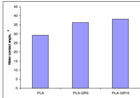
Figure 7: Water contact angles of the studied materials after weathering
