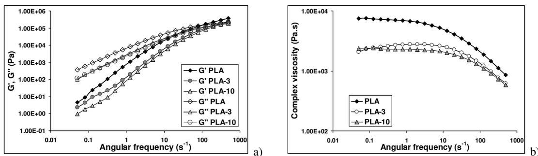
Figure 3: Variation of storage modulus and loss modulus (a), as well as complex viscosity (b) with angular frequency for PLA and PLA/grape seed composites
