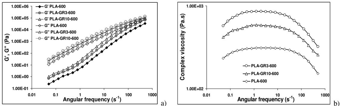
Figure 8: Variation of storage modulus and loss modulus (a), and complex viscosity (b) with angular frequency for PLA and PLA/grape seed composites after accelerated weathering
