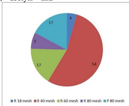
Figure 3: Particle size distribution of sawdust in % (R: retained, P: pass)
