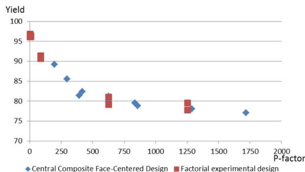
Figure 4: Fractionation yields of both experimental designs as a function of P-factor
