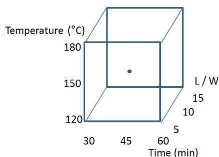
Figure 1:  $2^3$  Factorial design with time, temperature and liquid/solid ratio as variables
