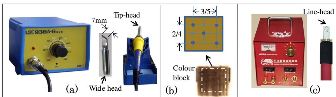
Figure 1: Controller and shape of its head for two electric soldering irons (a, c), and a sample of the color block with locations of 5 measurement points (b)
