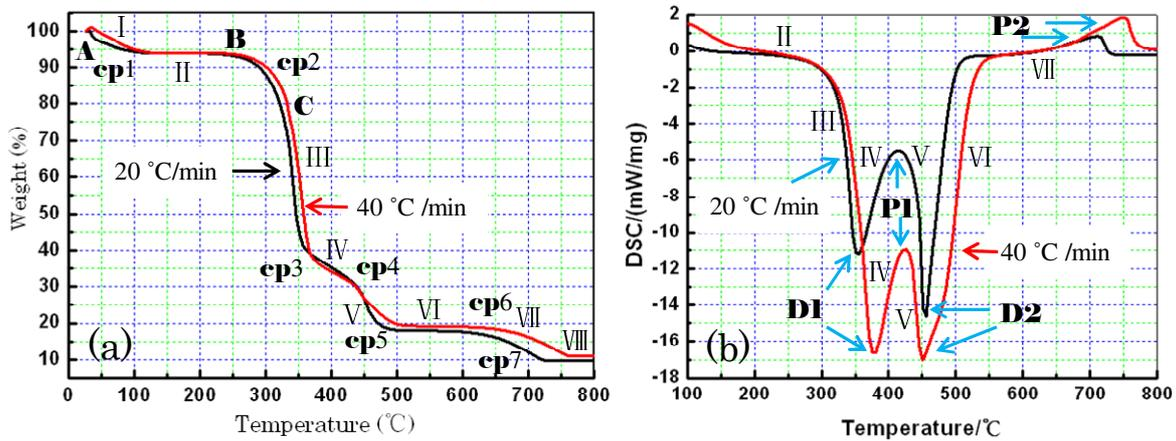
Figure 2: TG and DSC curves for paper samples
