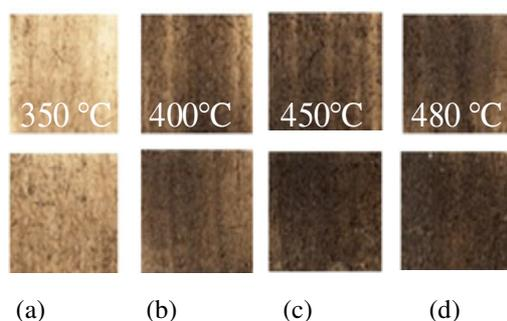
Figure 4: Color blocks generated by heat-induction
