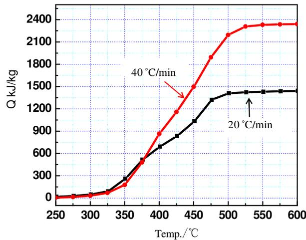
Figure 3: Endothermic curve of paper pyrolysis
