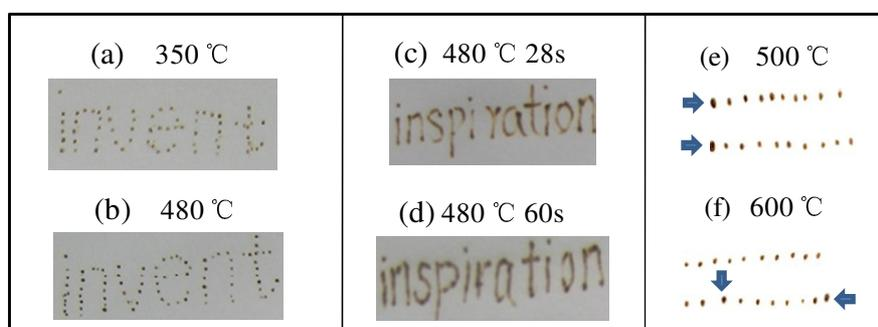
Figure 5: Simulation printing results at different temperatures by the print-click method (a, b, e, f), and scanning method (c, d)
