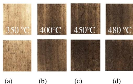
Figure 4: Color blocks generated by heat-induction
