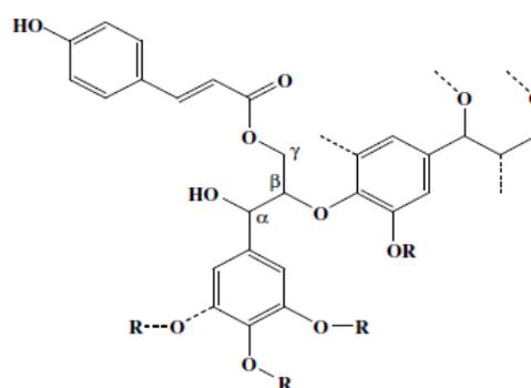
Figure 9: Representation of a coumarylated lignin fragment at  $\gamma$  position
