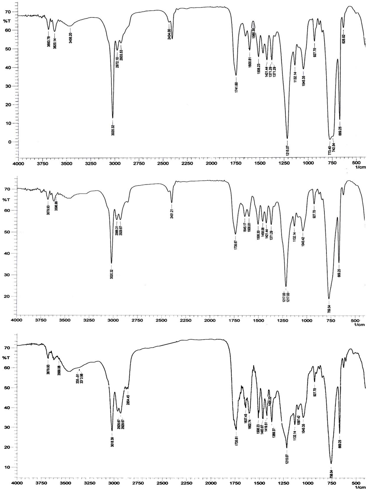
Figure 3: FT-IR spectra of acetylated lignins: a) LIG-Gly, b) LIG-DMF, c) LIG-Gly, DMF
