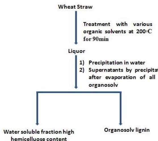
Figure 2: Scheme for isolation of lignin preparations obtained by treatment of wheat straw with organosolv
