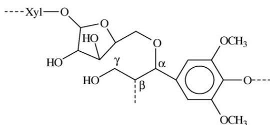
Figure 8: Direct attachment of arabinoxylyan to lignin (benzyl ether linkage)
