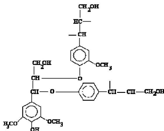
Figure 7: Simple representation of  $\alpha$ -aryl and  $\beta$ -aryl ether linkages
