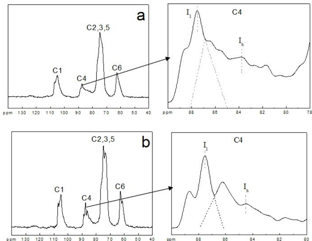
Figure 5: CP/MAS <sup>13</sup>C-NMR spectra of regenerated cellulose fiber in (a) dry and (b) wet state
