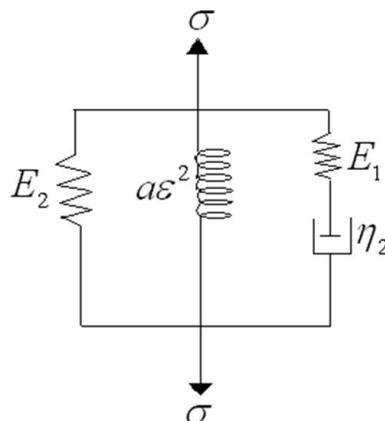
Figure 3: Non-linear viscoelasticity models for regenerated cellulose fiber in dry condition
