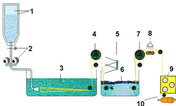
Figure 1: Scheme of multifilament spinning machine; 1 – a pressure extruder with a stainless cylinder having cooling jacket; 2 – gauging device; 3 – coagulation bath (12.5 wt% H<sub>2</sub>SO<sub>4</sub>/10 wt% Na<sub>2</sub>SO<sub>4</sub> aqueous solution, 20 °C); 4 – Nelson-type roller; 5 – water spray device; 6 – washing bath (hot water, 70 °C); 7 – post-drawing roller; 8 – post-treatment device (finishing oil bath); 9 – heating roller; 10 – take-up device
