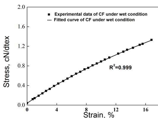
Figure 4: Experimental data and the fitted curve of regenerated cellulose fiber in wet condition
