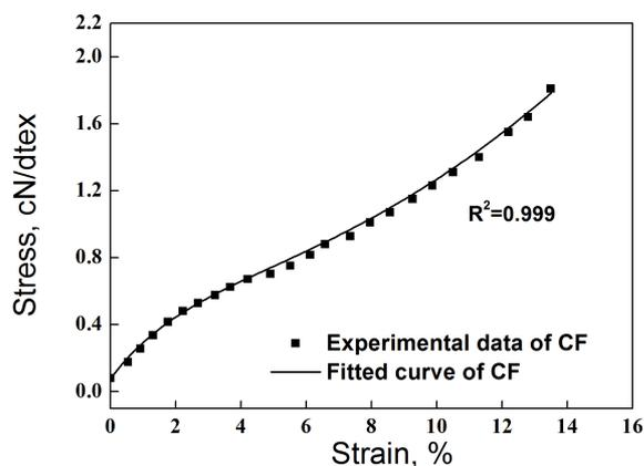
Figure 2: Experimental data and the fitted curve of regenerated cellulose fiber in dry condition
