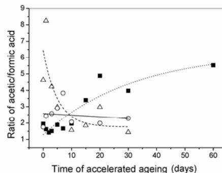
Figure 2: Influence of accelerated ageing at 98 °C and 50% RH on ratio of acetic/formic acids – (■) Sample A: control specimens, (Δ) Sample B: deacidified by dispersion of MgO, (○) Sample C: deacidified by mixture of MgO+MMMC (3:1)
