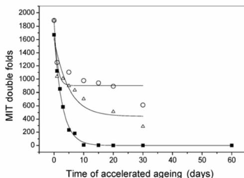
Figure 5: Decrease of folding endurance (MIT double folds) through accelerated ageing at 98 °C and 50% RH – (■) Samples A: control specimens, (Δ) samples B: deacidified by MgO dispersion, (○) samples C: deacidified by MgO+MMMC mixture (3:1)
