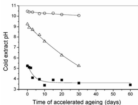
Figure 1: Influence of accelerated ageing at 98 °C and 50% RH on cold extract pH – (■) Sample A: control specimens, (Δ) Sample B: deacidified by dispersion of MgO, (○) Sample C: deacidified by mixture of MgO+MMMC (3:1)
