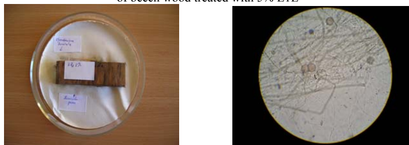
Figure 2: Macro- (left) and micro-images (right) of Humicola grisea on the surface of fir wood treated with 5% L1E
