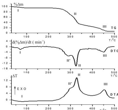
Figure 3: Representative wood thermograms (TG, DTG, SDTA) with dehydration and thermo-oxidation characteristics of hemicelluloses (II), cellulose (II), lignin (III)
