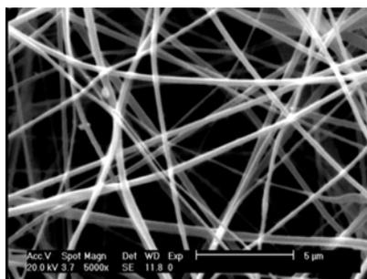
Figure 7: Electron micrograph of electrospun fibers at chitosan concentration of 10 wt%; 24 kV, 5 cm, TFA/DCM: 70/30
