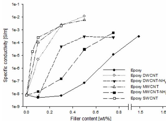
Figure 4: Electrical conductivity of nanocomposites as a function of filler content in weight percent<sup>97</sup>
