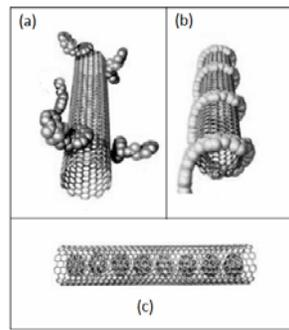
Figure 3: Non-covalent functionalization of CNTs by (a) surfactants, (b) wrapping, (c) the endohedral method
