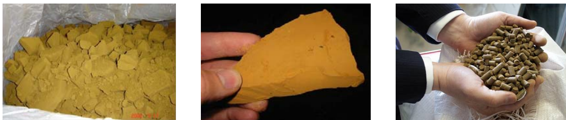
Figure 2: Lignin produced in the LignoBoost demonstration plant – filter cake and lignin pellets
