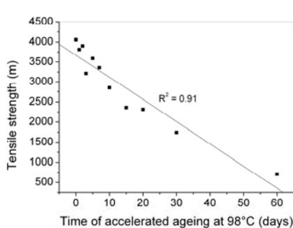
Figure 4: Influence of accelerated ageing on tensile strength at 98 °C
