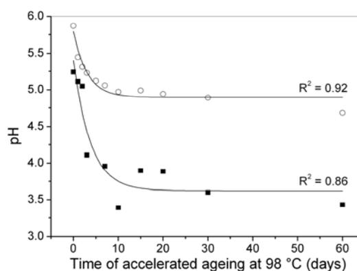
Figure 8: Influence of accelerated ageing on the surface and cold extract pH at 98 °C (○ – Surface pH; ● – Cold extract pH)
