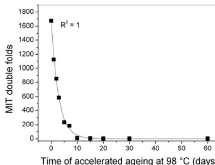
Figure 5: Loss of folding endurance (MIT double folds) under accelerated ageing at 98 °C
