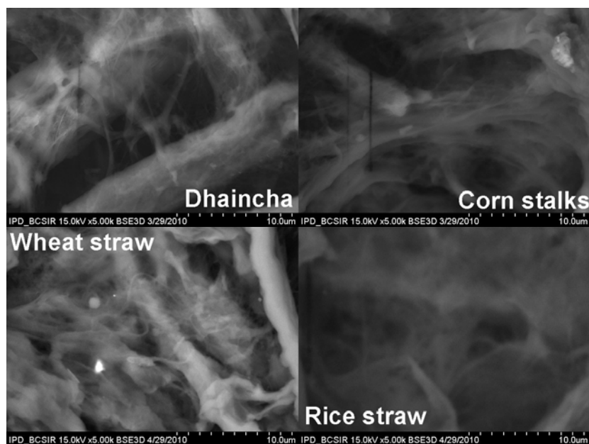
Figure 2: Extracted microfibrils from agricultural wastes (Magnification x5000)
