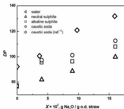
Figure 8: Degree of polymerization,  $DP$ , as a function of  $\text{Na}_2\text{O}$  charge
