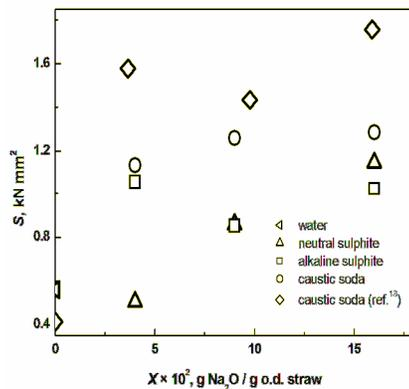
Figure 3: Influence of Na<sub>2</sub>O charge on bending stiffness,  $S$
