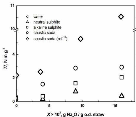
Figure 7: Tensile index,  $Tl$ , as a function of  $\text{Na}_2\text{O}$  charge
