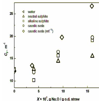
Figure 6: Curvature for tensile crack,  $C_F$ , as a function of  $\text{Na}_2\text{O}$  charge
