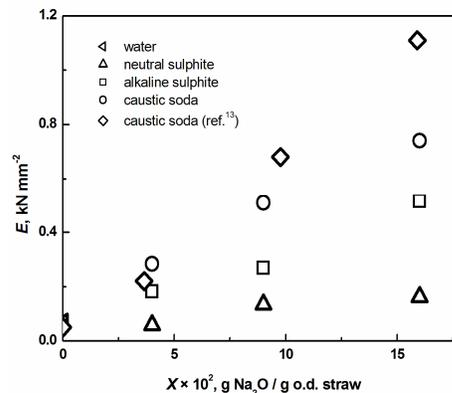
Figure 4: Influence of Na<sub>2</sub>O charge on bending modulus of elasticity,  $E$ , in the region of reversible deformation
