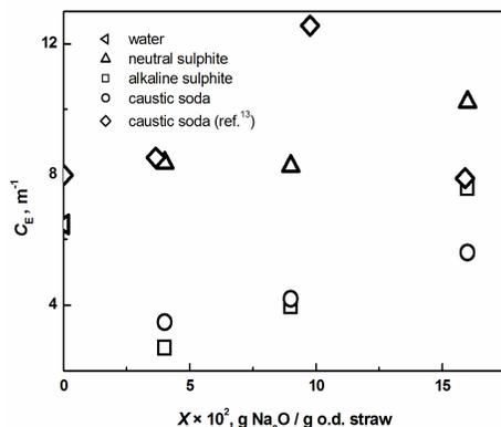
Figure 5: Maximum curvature,  $C_E$ , in the region of reversible deformation as a function of  $\text{Na}_2\text{O}$  charge
