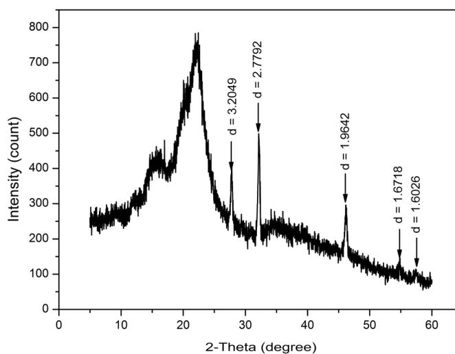
Figure 2: X-ray diffractogram of oxidized cellulose modified with Ag salt
