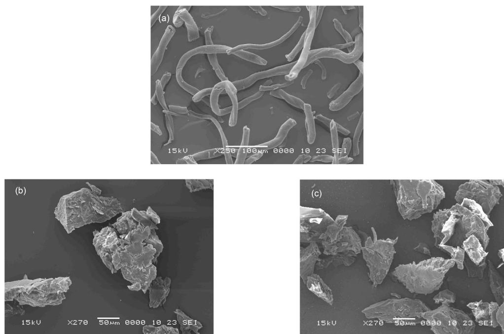
Figure 5: SEM images of (a) initial OC/Ag(I) and of the samples treated with (b) *C. albicans* in MEB (pH = 5.4) and (c) *S. epidermidis* in BHI (pH = 7.0) at 37 °C for 7 days
