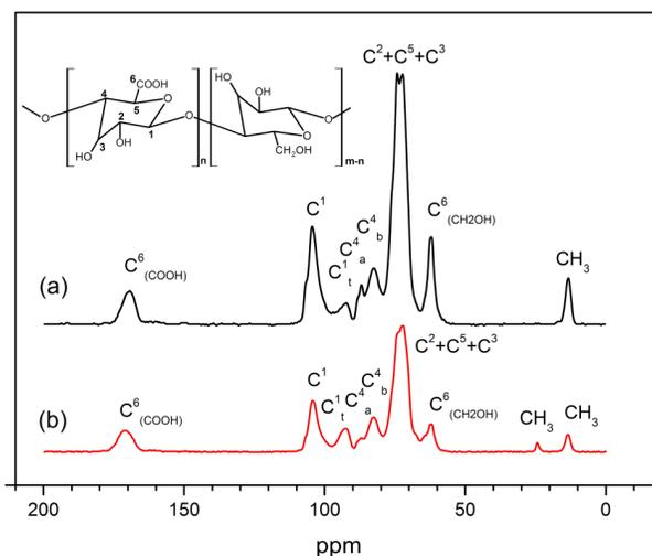
Figure 1:  $^{13}\text{C}$  CP/MAS NMR spectra of (a) oxidized cellulose and (b) oxidized cellulose with Ag salt
