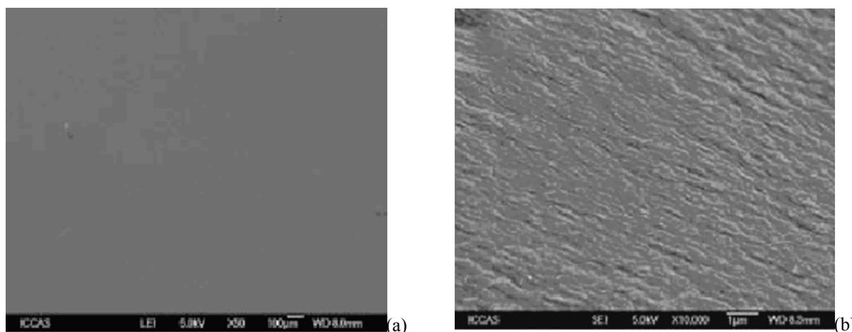
Figure 3: Scanning electron micrographs of (a) the surface and (b) cross-section of cellulose film loaded with 25 wt% turmeric powder
