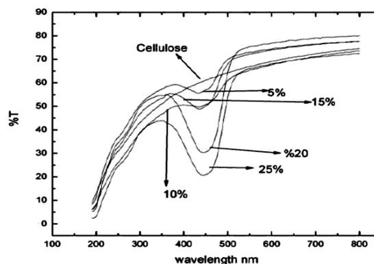
Figure 2: UV-visible spectra of cellulose/turmeric powder composite films
