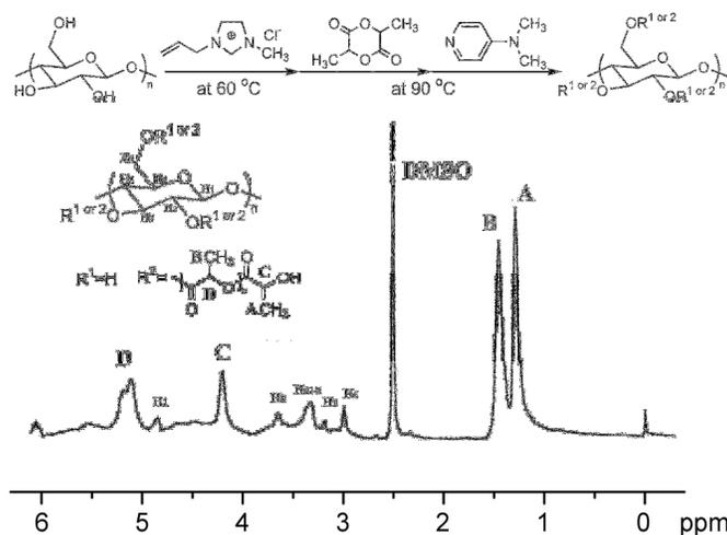
Figure 1:  $^1\text{H}$  NMR spectrum of cellulose-g-PLLA ( $\text{DP}_{\text{PLLA}}=3.15$ ) in  $\text{DMSO}-d_6$
