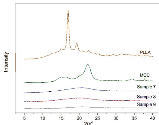
Figure 2: WAXD spectra of PLLA, MCC and cellulose-*g*-PLLA ( $DP_{\text{PLLA}} = 3.98$ ,  $DP_{\text{PLLA}} = 3.61$ ,  $DP_{\text{PLLA}} = 3.15$ )
