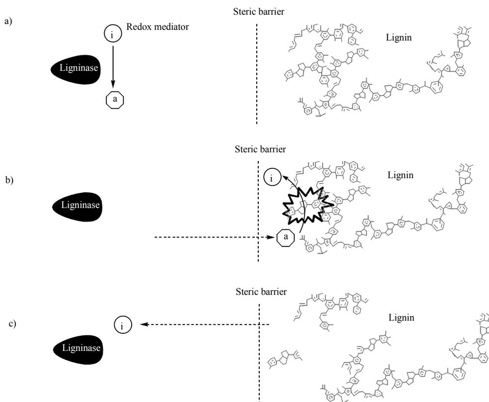
Figure 1: Principle of enzymatic lignin degradation by wood-degrading fungi: a) A lignin-modifying peroxidase oxidizes an inactive form of a redox mediator (i) to an active form (a); b) The active redox mediator can penetrate sterical barriers performing an unspecific lignin oxidation; c) The lignin gets fragmented in uncatalyzed reactions following oxidation. The redox mediator, now in inactive form, diffuses back to the lignin-modifying peroxidase for a new cycle
