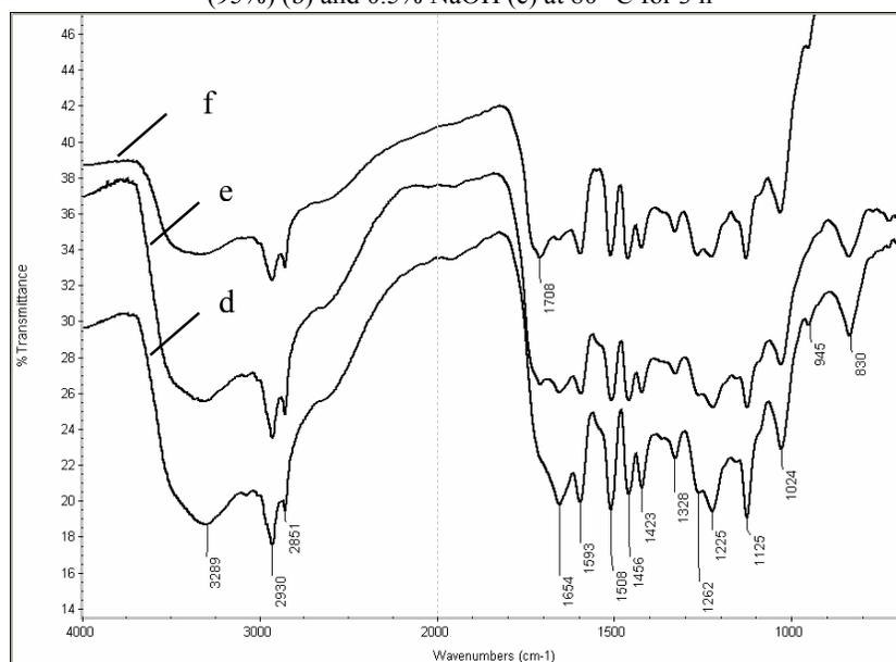
Figure 3: FT-IR spectra of *Carex meyeriana* Kunth lignin fractions isolated with 1% NaOH (d), 1.5% NaOH (e) and 2% NaOH (f) at 80 °C for 3 h
