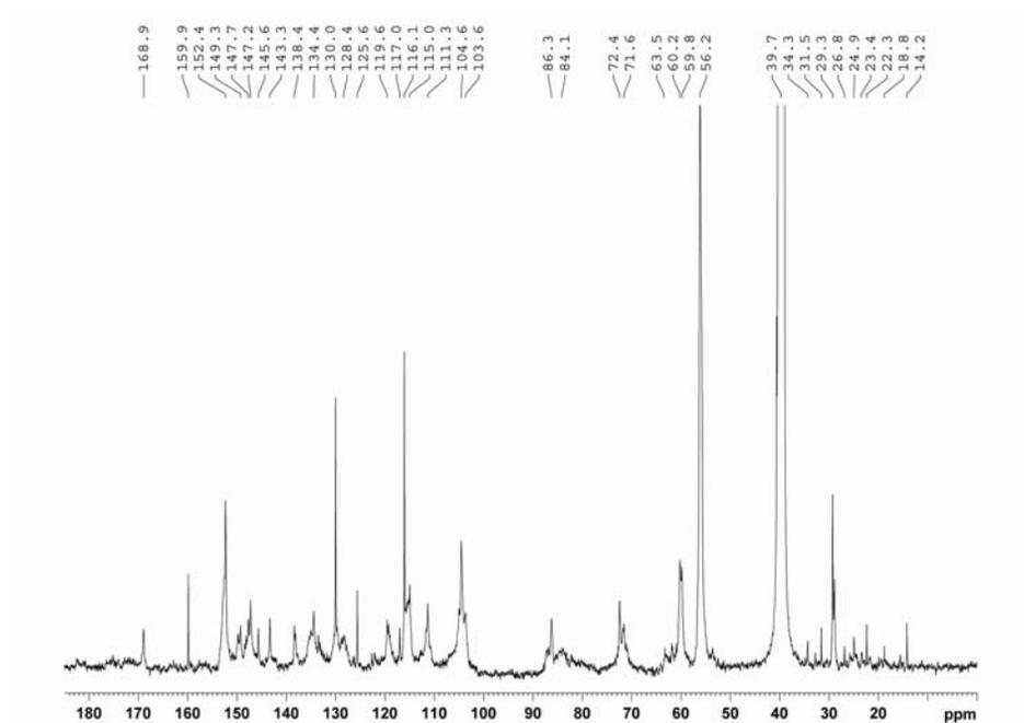
Figure 7:  $^{13}\text{C}$  NMR spectrum of lignin fraction L3 isolated with 0.5% NaOH at 80 °C for 3 h
