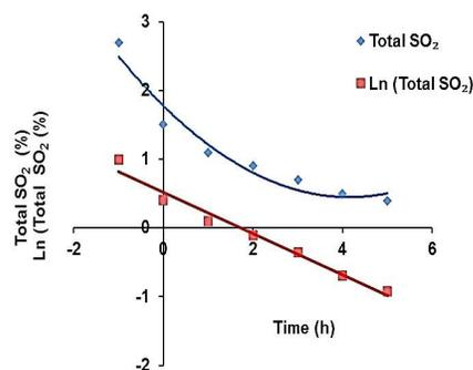
Figure 3: Total SO<sub>2</sub> and the logarithmic value of the total SO<sub>2</sub> for the cooking experiment shown in Figure 2. As the logarithmic correlation is linear, the chemical reaction can be assumed to be of first order with respect to total SO<sub>2</sub>
