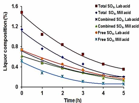
Figure 2: Total SO<sub>2</sub>, combined SO<sub>2</sub> and free SO<sub>2</sub> levels in laboratory experiments where either mill-prepared or lab-prepared cooking acid was used. The initial composition of the cooking acids was always: Total SO<sub>2</sub> 2.7%, combined SO<sub>2</sub> 1.5% and free SO<sub>2</sub> 1.2%, calculated as SO<sub>2</sub>; L/W-ratio 4.6; base content 5%, calculated on the weight of dry wood chips and as Na<sub>2</sub>O; temperature 154 °C
