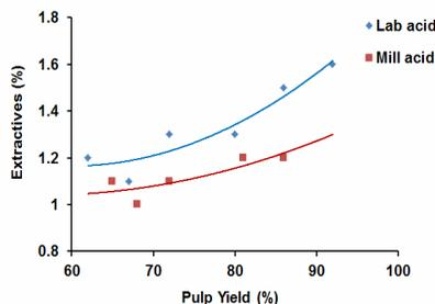
Figure 8: Acetone extractives content in the pulp during bisulphite cooking of spruce with a lab-prepared and a mill prepared cooking acid
