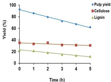
Figure 4: Bisulphite cooking of spruce with a laboratory-prepared cooking acid. Conditions used: total  $\text{SO}_2$  2.7%, combined  $\text{SO}_2$  1.5% and free  $\text{SO}_2$  1.2%, calculated as  $\text{SO}_2$ ; base charge 5%, calculated as  $\text{Na}_2\text{O}$  and on dry chips; temperature 154 °C. Note that time zero was defined as the time when full cooking temperature was reached, which means that the time when the autoclaves were mounted into the digester was “minus 2 h”
