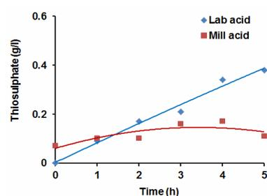
Figure 7: Thiosulphate content in the cooking liquor during bisulphite cooking of spruce with lab-prepared or mill-prepared cooking acids. The lower thiosulphate number for the mill-prepared acid experiments was probably due to more lignin condensation reactions, which reduced the thiosulphate content in the free liquor phase
