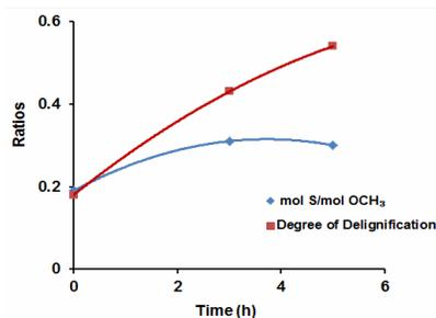
Figure 6: Degree of sulfonation measured as mol S/mol  $\text{OCH}_3$  and the degree of delignification during bisulphite cooking of spruce (temperature 154 °C)
