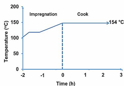
Figure 1: Temperature profile during the laboratory cooks; cooking temperature: 154 °C;
