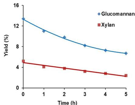
Figure 5: Glucomannan and xylan contents in the pulp during bisulphite cooking of spruce with lab-prepared cooking acid. The temperature was 154 °C. Time zero was defined as the time when full cooking temperature was reached and the time when the autoclaves were mounted into the digester was “minus 2 h”
