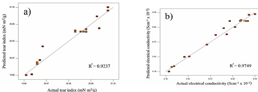
Figure 1: Comparison between the actual and experimental values for a) tear index b) electrical conductivity
