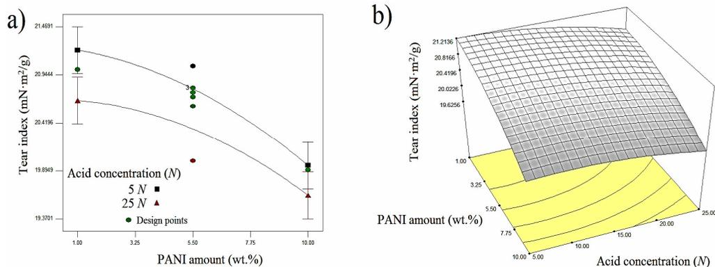
Figure 2: 2D and 3D response surface plot for tear index
