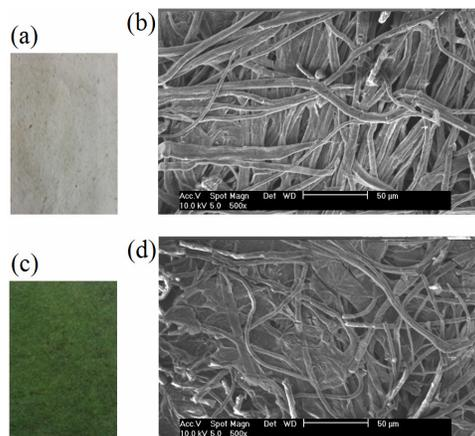
Figure 4: Photographs and electron micrographs of (a-b) unmodified KF paper, (c-d) optimized KF-PANI paper
