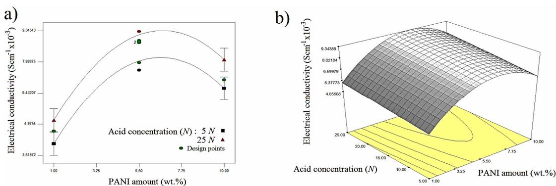
Figure 3: 2D and 3D response surface plot for electrical conductivity
