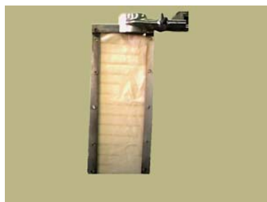
Figure 1: Mostashari's Flammability Tester with a treated fabric inserted and pinned in its internal splits, prior to the fulfillment of the flammability test
