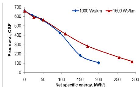
Figure 1: Evolution of freeness with pulp refining
