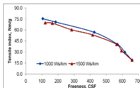
Figure 7: Effect of pulp freeness on tensile index
