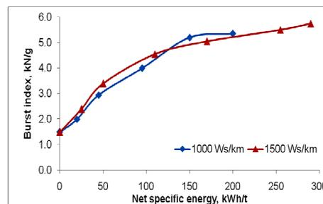
Figure 9: Evolution of burst index with pulp refining
