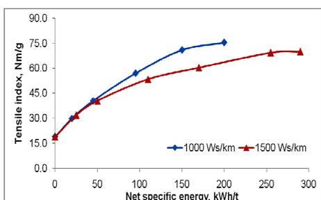
Figure 6: Evolution of tensile index with pulp refining
