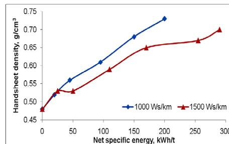
Figure 5: Evolution of handsheet density with pulp refining
