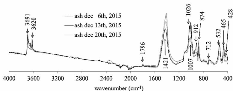
Figure 2: FT-IR spectra of the ash obtained from three weekend supplement samples by burning at 420  $^{\circ}\text{C}$  (prominent bands are indicated)
