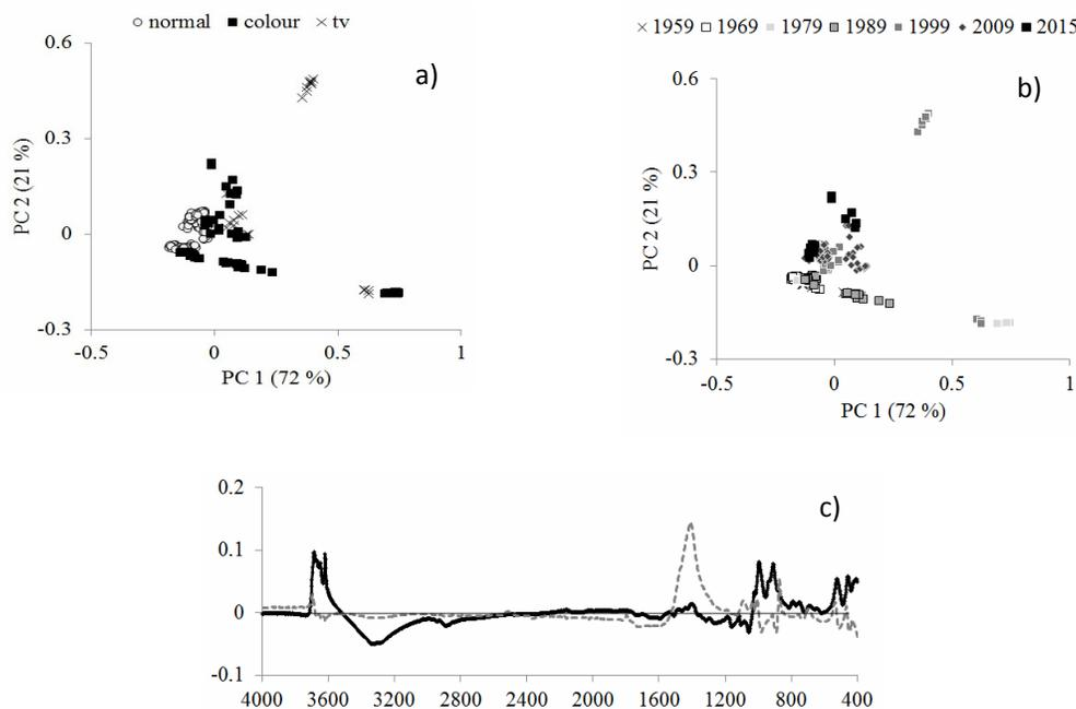
Figure 1: PCA based on infrared spectra (4000-400  $\text{cm}^{-1}$ ) of all archive samples  $n=223$ : Scores plots with PC 1 and PC 2 marked a) according to the type of paper, b) according to the year; c) loadings plot of PC 1 and PC 2
