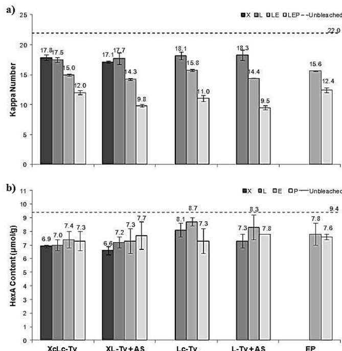
Figure 2: Evolution of kappa number (a) and hexenuronic acid content (b) after each stage in biobleaching sequences with xylanase pretreatments and their respective controls
