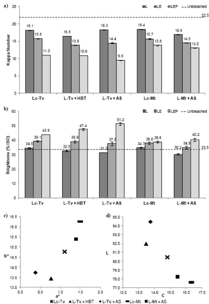
Figure 1: Evolution of pulp properties after each stage in biobleaching sequences: kappa number (a); brightness (b) and color coordinates of biobleached pulps: CIE  $L^*a^*b^*$  (c) and CIE  $L^*C^*$  (d)
