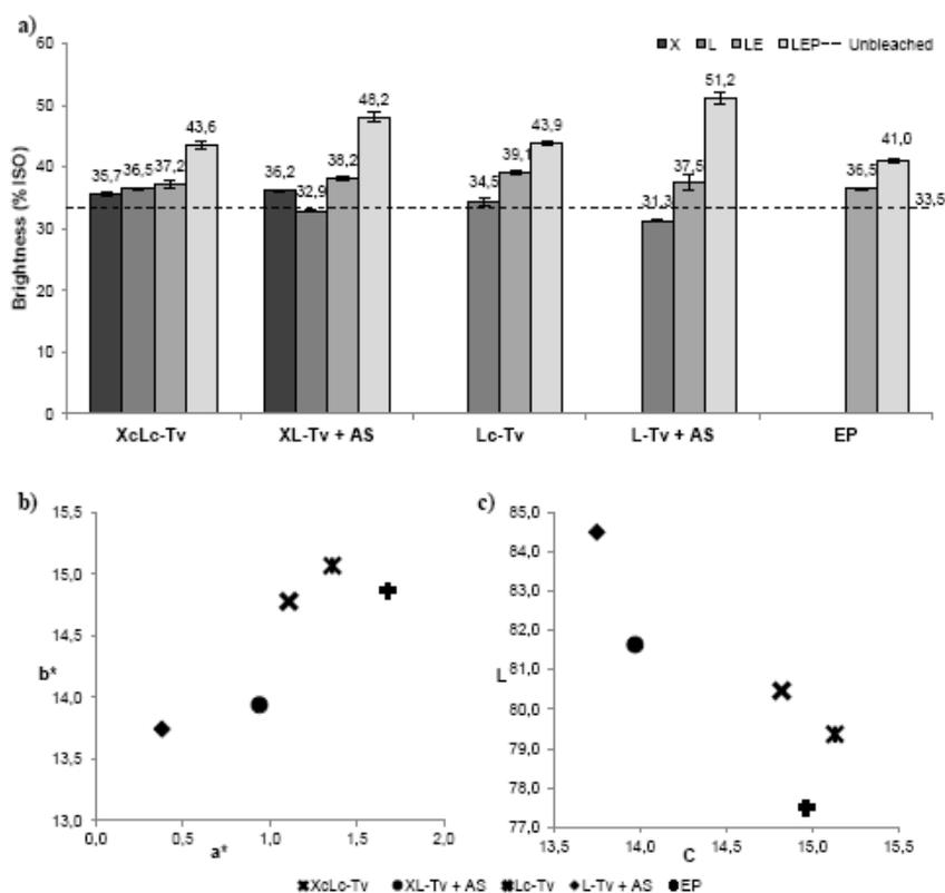
Figure 3: Evolution of brightness after each stage in biobleaching sequences with xylanase pretreatments and their respective controls (a)
