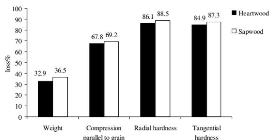
Figure 1: Mean reduction values of weight and mechanical strength
