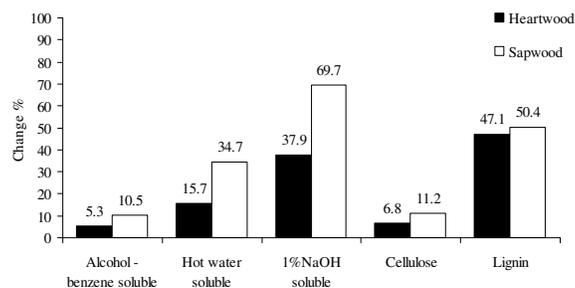
Figure 2: Mean reduction values of chemical components
