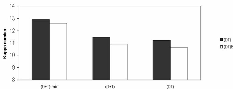
Figure 3: Effects of different mixing of bleaching agents. See materials and method for mixing conditions.
