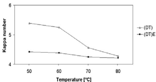
Figure 1: Effect of temperature on (DT)-bleaching of oxygen delignified mixed softwood kraft pulp (pH – 4.5, incubation time – 45 min)
