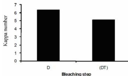
Figure 2: D stage compared to (DT) stage on oxygen delignified hardwood kraft pulp
