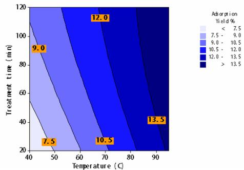
Figure 5: Interactive effect of temperature and time on adsorption yield (fiber consistency: 4.1%; ratio of extracts to fiber: 2.6)
