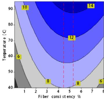
Figure 2: Interactive effects of fiber consistency and adsorption temperature on adsorption yield (extract ratio to fiber: 2.1; time: 70 min)
