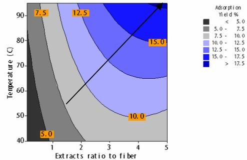
Figure 3: Interactive effects of extracts-to-fiber ratio and adsorption temperature on adsorption yield fiber consistency: 4.1%; time: 70 min)
