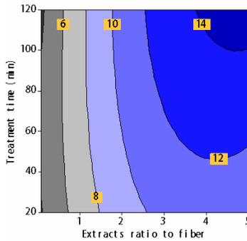
Figure 4: Interactive effects of extract ratio and treatment time on adsorption yield (fiber consistency: 4.1%; adsorption temperature: 67.5 °C)
