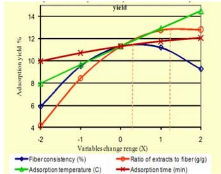
Figure 1: General profile of all process factors on adsorption yield
