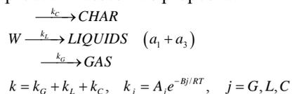
where  $k_i$  are rate constants for gas (G), liquid (L) and char (C) formation,  $A_j$  is the pre-exponential factor,  $B_j$  – activation energy,  $R$  – gas constant,  $T$  temperature and  $a_i$  – stoichiometric coefficients.
