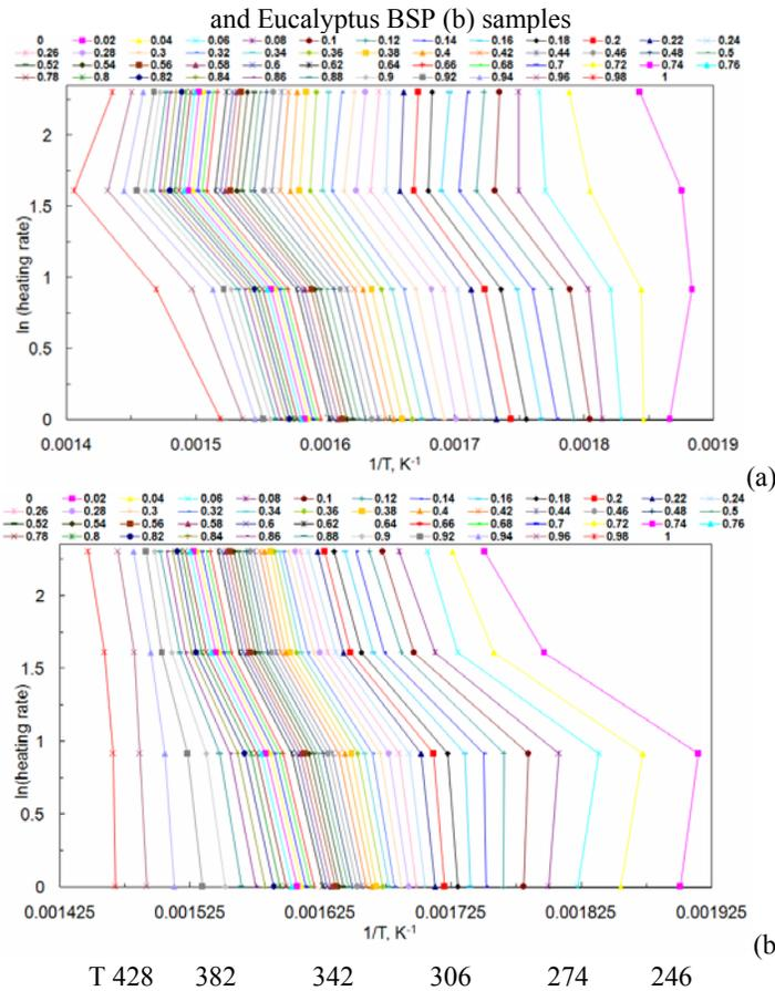
Figure 7: Flynn-Wall graphs corresponding to the second thermogravimetric step for Eucalyptus chips (a) and Eucalyptus BSP (b), at heating rates of 1, 2.5, 5, 10 °C/min
