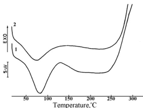
Figure 1: DSC curves in the region of water desorption and low molecular weight compounds loss; 1 – *Eucalyptus* chips; 2 – *Eucalyptus* BSP
