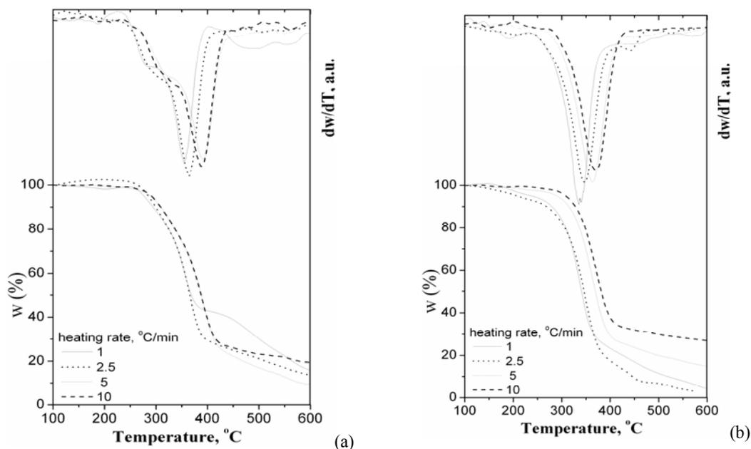
Figure 3: TG/DTG curves of *Eucalyptus* chips (a) and *Eucalyptus* BSP (b), recorded at different heating rates
