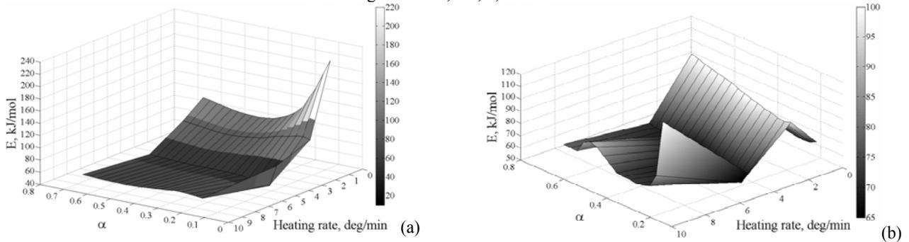
Figure 8: Dependence of activation energy on heating rate and conversion degree for Eucalyptus chips (a) and Eucalyptus BSP (b) samples
