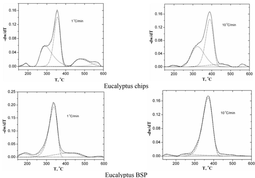
Figure 4: Deconvoluted DTG curves recorded at heating rates of 1 °C/min and 10 °C/min for Eucalyptus chips and Eucalyptus BSP samples
