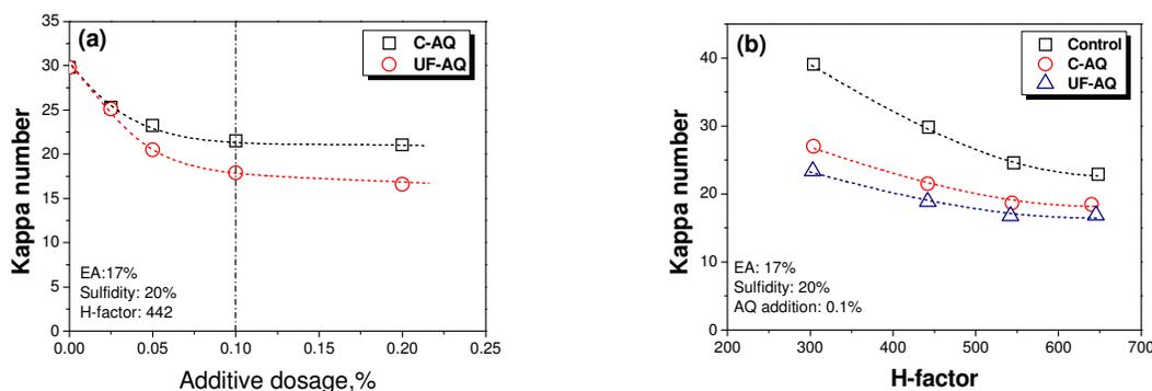
Figure 3: Kappa number variation as a function of (a) additive dosage; (b) H-factor
