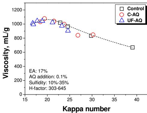
Figure 6: Variation of pulp viscosity as a function of kappa number
