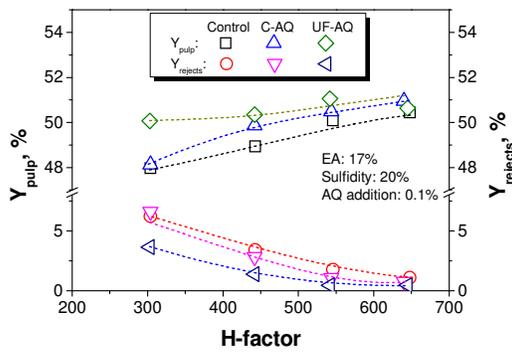
Figure 4: Variation of screened pulp yield ( $Y_{pulp}$ ) and screened reject yield ( $Y_{rejects}$ ) as a function of H-factor
