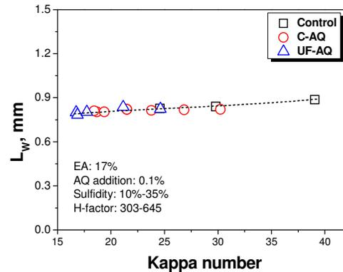
Figure 7: Variation weighted average fiber length ( $L_w$ ) as a function of kappa number
