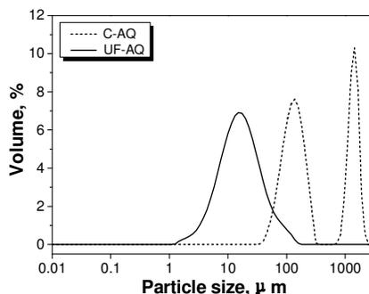
Figure 2: Particle size distributions of C-AQ and UF-AQ
