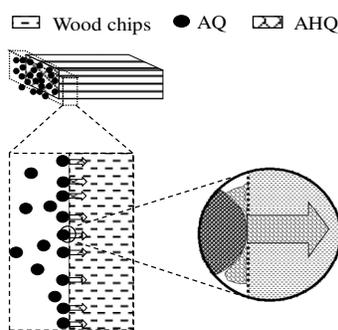
Figure 1: AQ mass transfer mechanism during alkaline pulping
