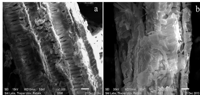
Figure 2: Scanning electron micrographs of (a) native and (b) SAMAP biomass (magnification: 1,000X)
