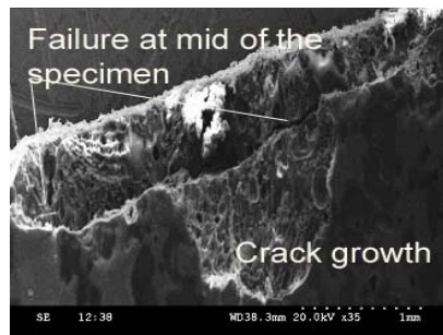
Figure 4: SEM images of fracture surfaces after (a) tensile, (b) flexural and (c) impact testing
