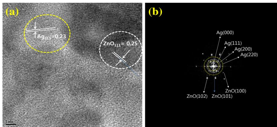
Figure 7: (a) HR-TEM image of Ag-ZnO nanocomposite showing the lattice fringes of Ag and ZnO and (b) combined SAED pattern of Ag/ZnO (5:5) nanocomposite
