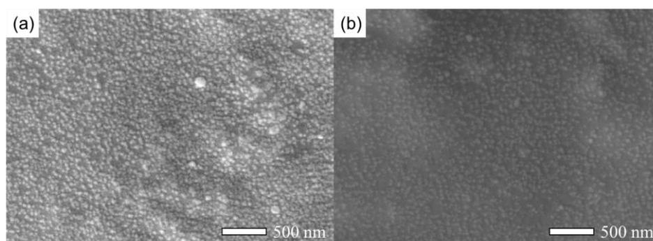
Figure 9: SEM images of cotton/ZnO (5:5) (a) before washing of cotton/ZnO and (b) after washing of cotton/ZnO
