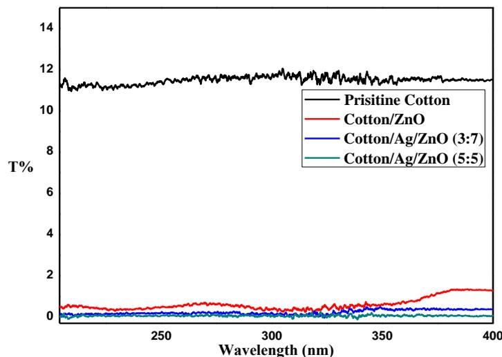
Figure 8: UV-vis transmittance spectra of pristine cotton, cotton/ZnO, cotton/Ag/ZnO (3:7) and cotton/Ag/ZnO (5:5)
