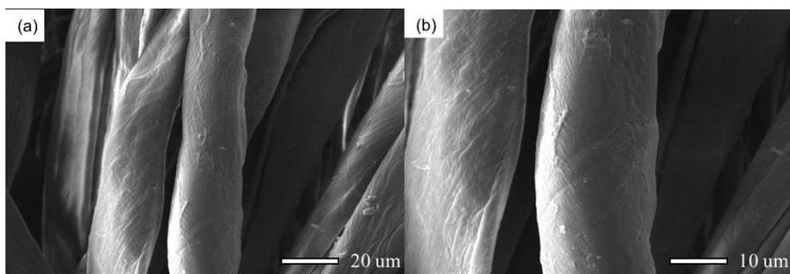
Figure 2: SEM images of pristine cotton at magnifications of (a) 3000 $\times$  and (b) 5000 $\times$
