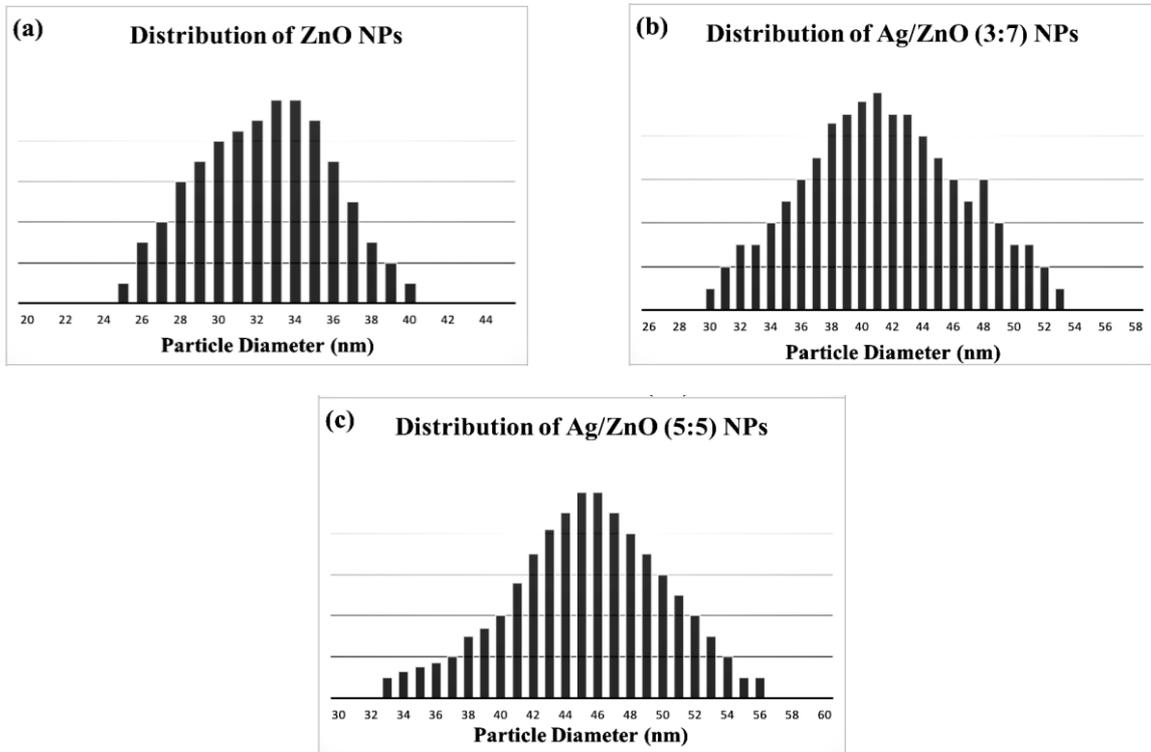
Figure 6: Particle size distribution of (a) ZnO NPs, (b) Ag/ZnO (3:7) NPs, and (c) Ag/ZnO (5:5) NPs
