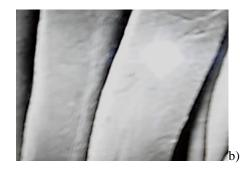
Figure 3: Micrographs of a) control fabric bleached at 95 °C without ultrasound; b) fabric subjected to ultrasound assisted bleaching at room temperature for 90 min (x1540)
