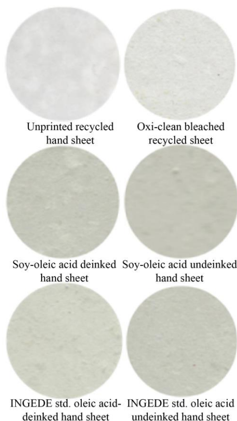
Figure 5: Surface images of undeinked and deinked handsheets
