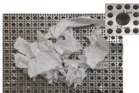
Figure 4: Screen for separation of pulp fibers and plastic coating
